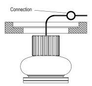
Remove bezel and gasket by using the supplied allen key to unscrew the 3 CSK screws.
