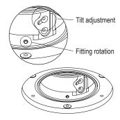
8 Once adjusted to the desired position, replace the gasket and bezel.
